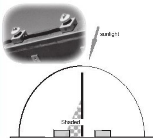
Figure 3. The solar sensors are located above the target board. When a cell becomes shaded, the Q-Trac motor automatically adjusts to maintain the device's alignment.
