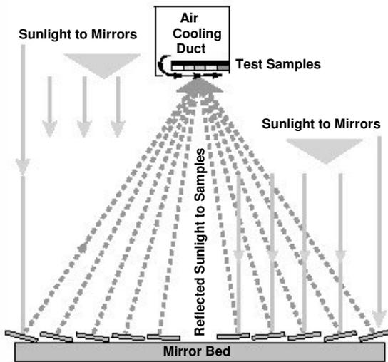
Figure 1. The Q-Trac is a Fresnel concentrator. The sunlight is Reflected and concentrated by the 10 mirrors directly to the target board.
